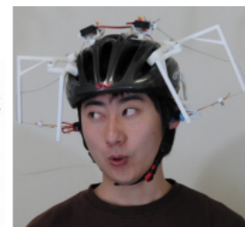
Fig. 7: Navigation by ear pulling as proposed by Kojima et al. 12 showing the 3-dimensional approach (left) and the device (right).
