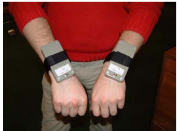
Fig. 3: Navigation bracelets on the left and right hand as used by S. Bosman et al. 5
